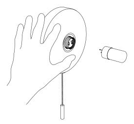
8. Carefully slide the Glass Globe over the Lightbulb, thread the Globe onto the Tech Assembly, and tighten it to the desired orientation. The rubber will allow for small adjustments to orientation, but care must be taken not to overtighten. Loosening the Globe might in some cases be the best way to achieve the desired orientation.
