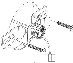
5. Connect one wire from the Pull Chain Switch to the hot wire on the Socket Assembly and the other wire from the switch to the junction box hot wire.
