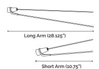
3. Then, insert the two rods of the LONGER arms into the top holes of the Centering Block. The LONGER arms of the Pendant should angle upward when installed. The last arm will require a bit more effort to insert as it is the final component of the tensegrity structure.
