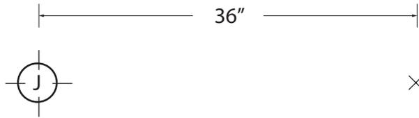
3. Unscrew top of Aircraft Cable Support apart from bottom, and put bottom aside. If using Drywall Anchor, install Anchor in ceiling on mark. Next, install top of Aircraft Cable Support by driving Drywall Screw through hole on top of Aircraft Cable Support into mark on ceiling so that Aircraft Cable Support sits tightly against ceiling.
