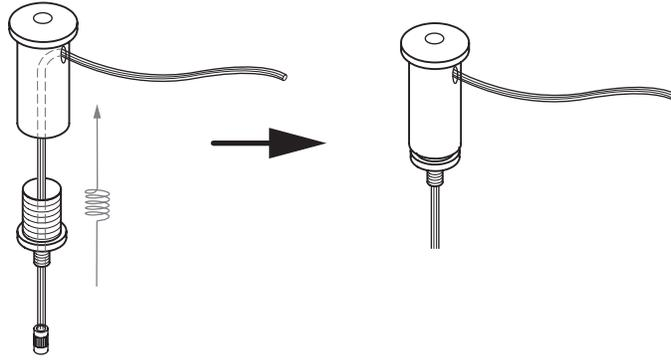
10. Adjust fixture height by increasing/decreasing drop of Aircraft Cable by pushing up on threaded nipple on bottom of Aircraft Cable Support and pulling/pushing Aircraft Cable through side hole until fixture hangs level.
