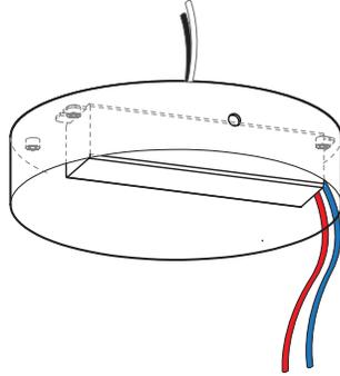
2. Determine axis of orientation of fixture. On this axis, draw a mark on ceiling 36" from the center of your junction box. This mark will act as the center for your Aircraft Cable Support.
