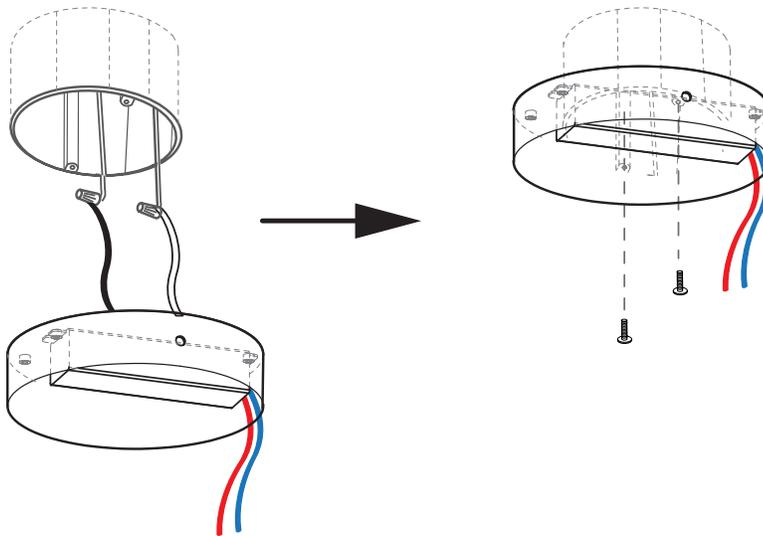
6. Pull cord from Beam Pendant through Strain Relief and Canopy. Determine the hanging length of your fixture by positioning assembled fixture in desired location. Once height has been determined tighten the Strain Relief set screw. Cut excess cord and strip wire ends.
