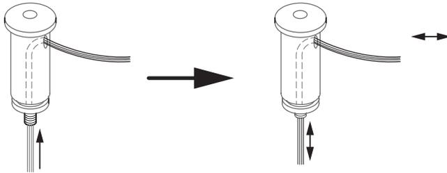
11. When fixture is level, attach screw cap to threaded nipple on Aircraft Cable Support tightly. Trim excess Aircraft Cable. Turn the fixture on, and enjoy!
