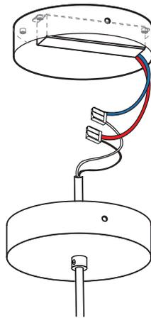
8. Slide Canopy over Fire Enclosure. Align holes on side of Canopy with holes on side of Fire Enclosure. Secure Canopy to Fire Enclosure by tightening Thumb Screws through Canopy into holes in Fire Enclosure tightly.
