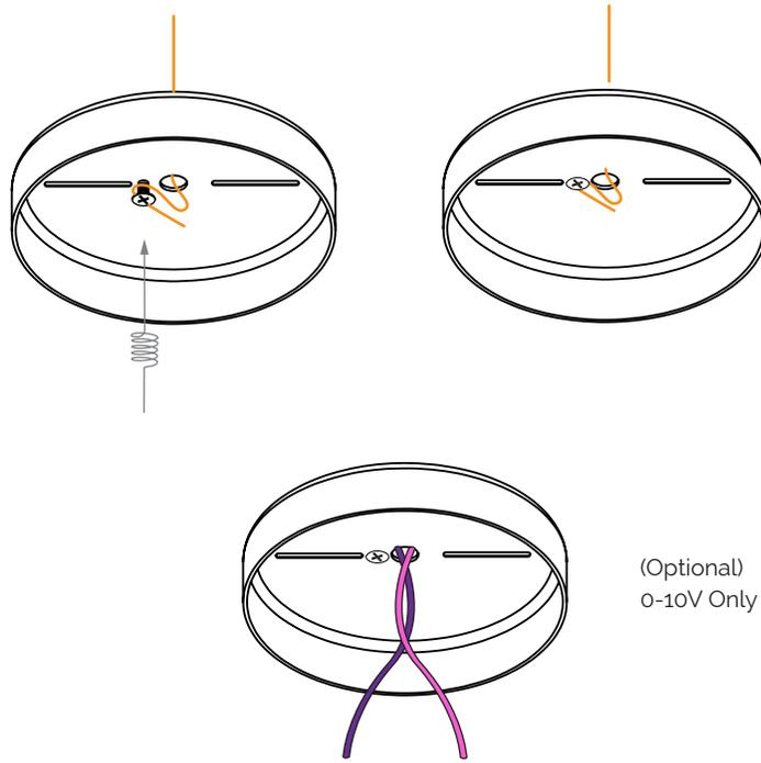
5. Connect the AC Input leads (black, white) to power source with Wire Nuts. Next, install Fire Enclosure to junction box with Mounting Screws.
