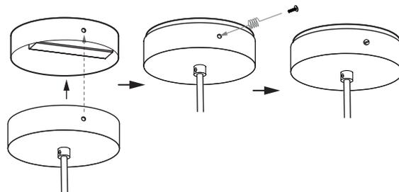
9. Separate Aircraft Cable Support by unscrewing the screw cap and the bottom of the cable support body. Pull Aircraft Cable from fixture through screw cap and both bottom and top of the Aircraft Cable Support, then out through side hole. Thread Aircraft Cable Support bottom into the top, pushing down on threaded nipple slightly to allow wire to freely spin.
