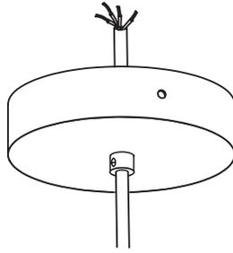
7. Isolate DC Output wires from each driver. Connect Wire from fixture to Driver one at a time as follows:
